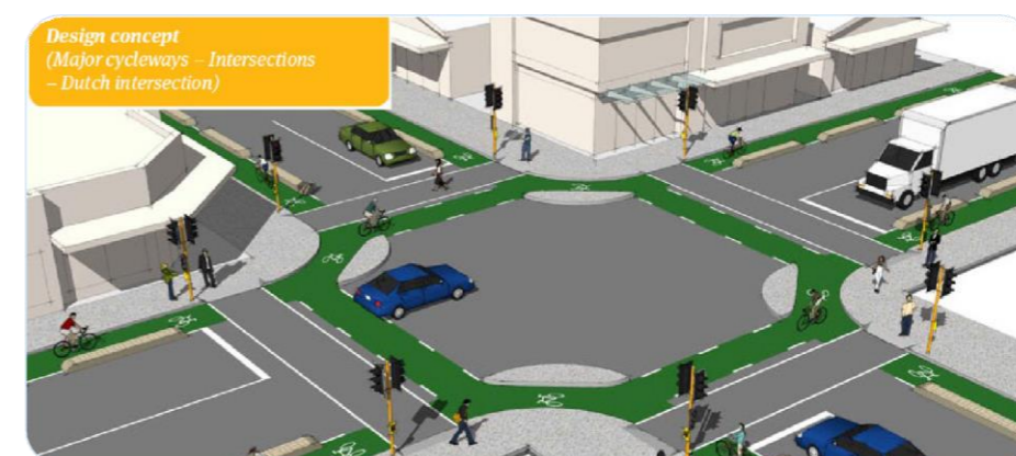
Figure 16: Key Infrastructure Elements of Protected Junction
